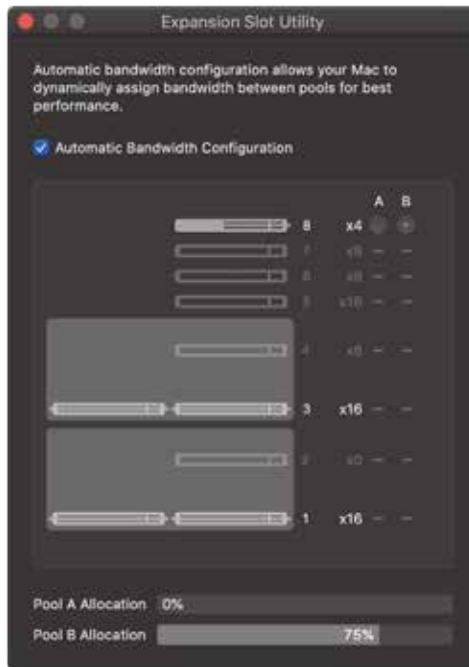
Expansion Slot Utility showing two MPX Modules installed, represented by the gray boxes, and the default Automatic Bandwidth Configuration selected.
